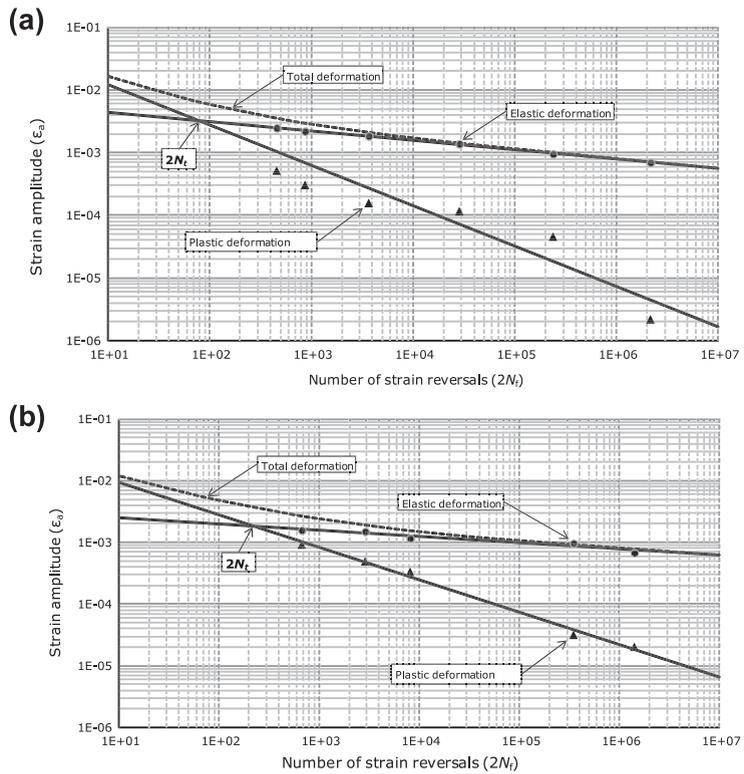
Fig. 8. Strain–life curves at (a) RT, (b) 500 °C, (c) 600 °C and (d) 700 °C.
