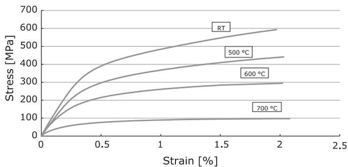
**Fig. 4.** Compression stress–strain curves at RT, 500 °C, 600 °C and 700 °C.
