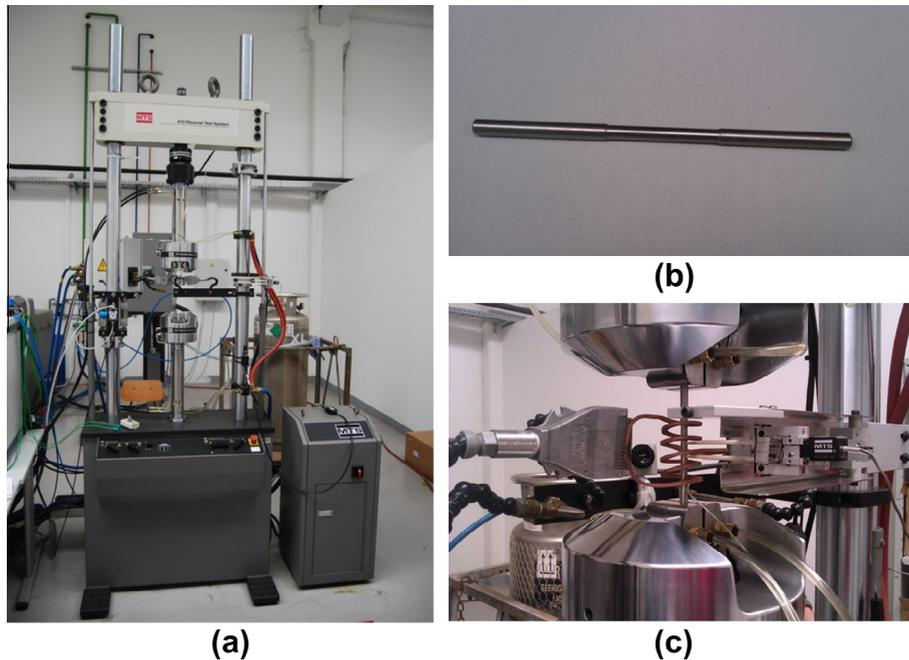
**Fig. 2.** Material testing machine MTS 810 (a), test specimen (b), induction heater and MTS ceramic extensometer (c).
