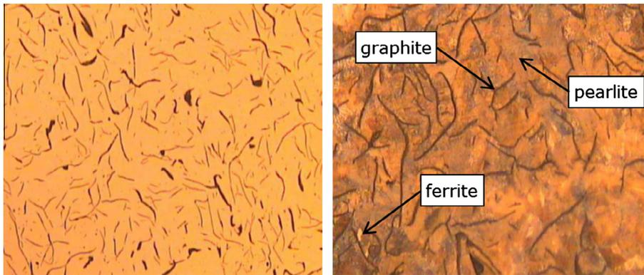
**Fig. 1.** Microstructure of the material at RT; left: un-etched, 100 $\times$ ; right: etched, 200 $\times$ .
