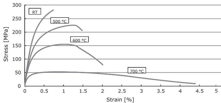
**Fig. 3.** Tensile stress–strain curves at RT, 500 °C, 600 °C and 700 °C.
