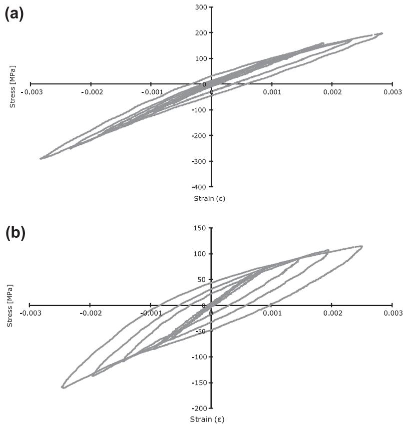
Fig. 7. Stress–strain hysteresis loops at (a) RT, (b) 500 °C, (c) 600 °C and (d) 700 °C.
