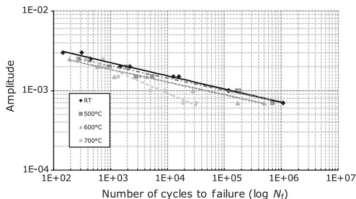
**Fig. 5.** Number of cycles to failure as a function of amplitude loading.
