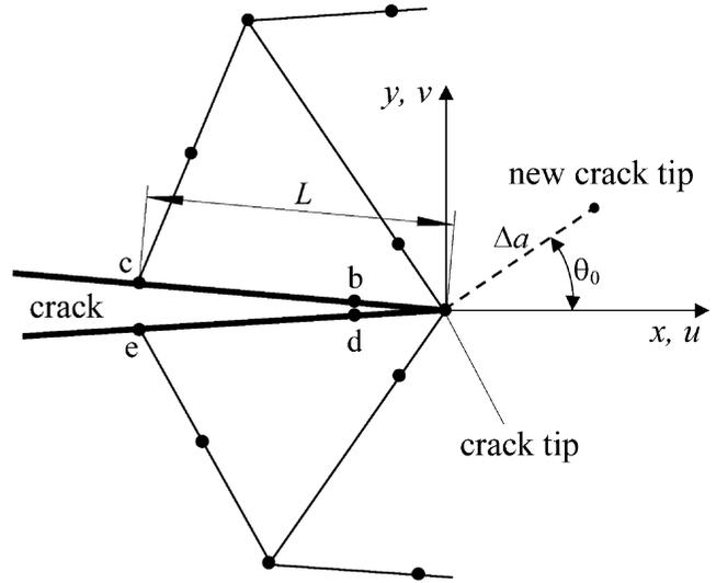
Fig. 5. Triangular quarter-point elements around crack tip.
