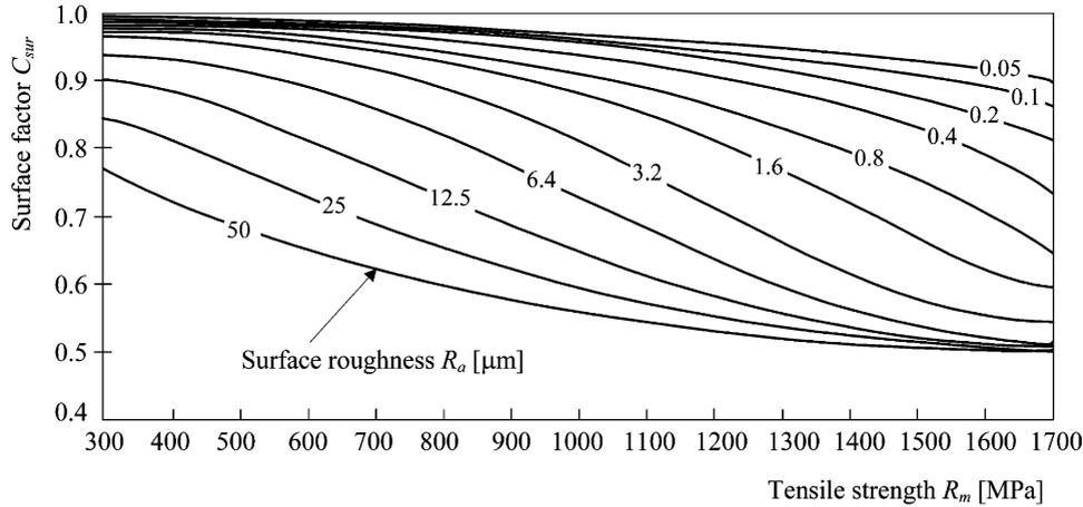
Fig. 4. Surface finish correction factor  $C_{sur}$ .
